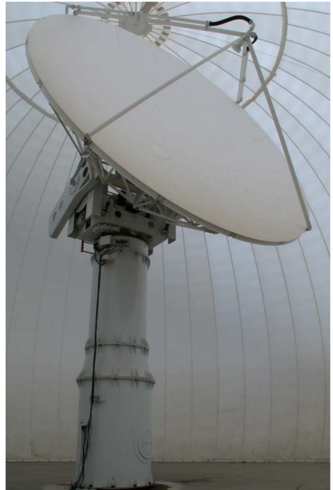
CSU-CHILL's 9-meter dual-polarized S-band Antenna
