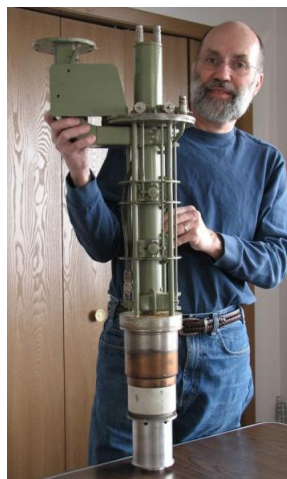
Figure 10: CSU-CHILL Senior Electrical Engineer David Brunkow describes the construction features of a VA-87B Klystron microwave power amplifier tube during a virtual tour of the Facility.
